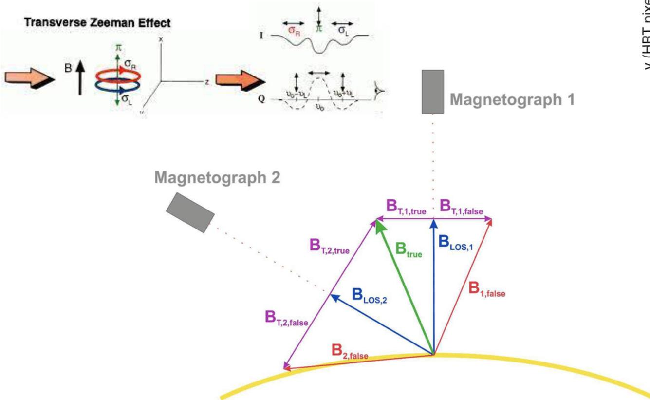
The **Stereoscopic Disambiguation Method (SDM)** that solves the 180-degree ambiguity by combining information from two vantage points: SO/PHI, SDO/HMI.
