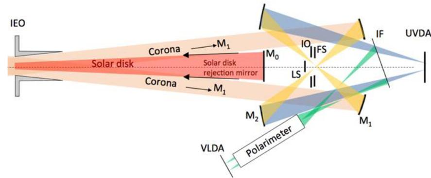
Metis is an externally-occulted coronagraph designed to provide full imaging of the extended corona ( $\sim 1.7-9 R_{\odot}$ ) in:
