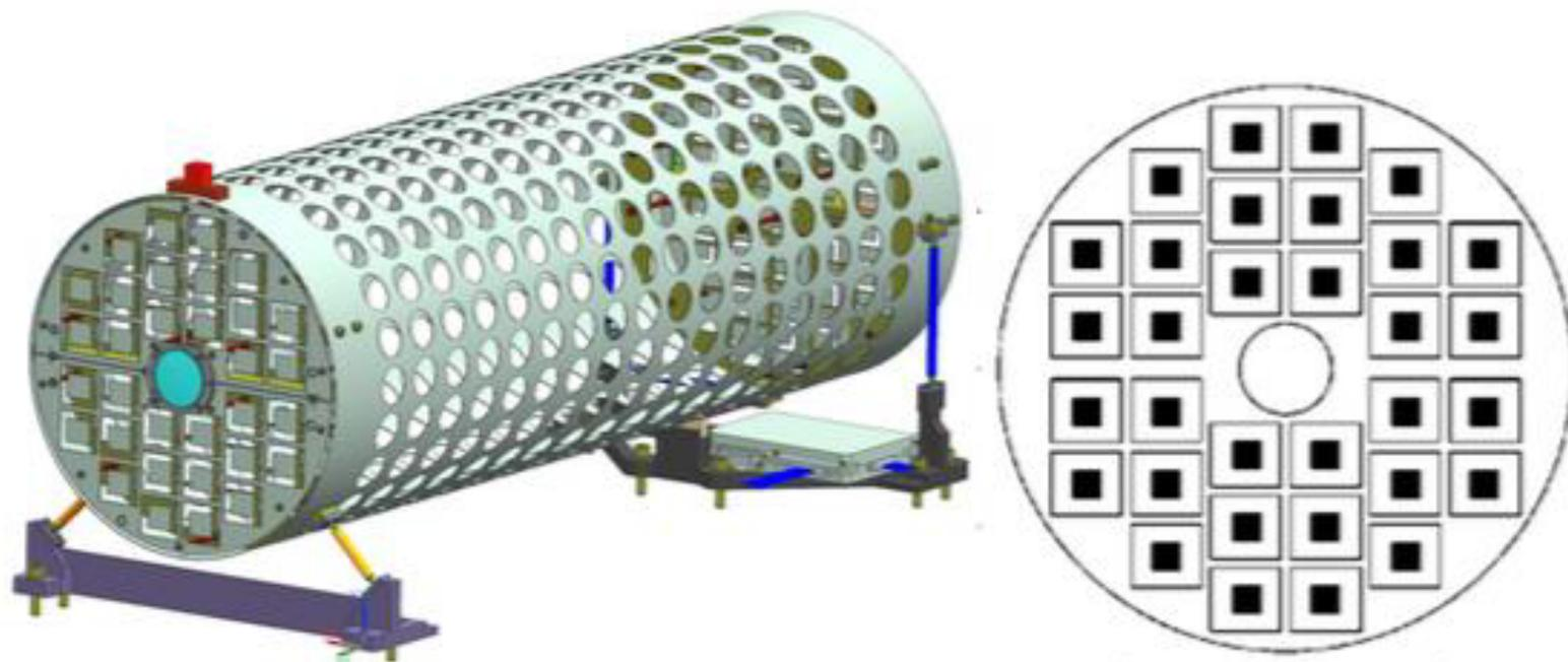
Figure 4. *Left:* The STIX Imager. *Right:* Layout of the front grid assembly. Its 180 mm diameter contains thirty-two 22 mm  $\times$  20 mm subcollimators (open rectangles) as well as room for an aspect lens at its center. The rear grid assembly is similar except that there is no lens and the subcollimators dimensions are only 15 mm  $\times$  15 mm. The solid squares represent the 10 mm  $\times$  10 mm<sup>2</sup> detectors located in the DEM behind the grids.
