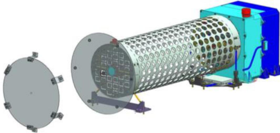
Since the use of focusing optics to achieve arcsec-class imaging over the 4-150 keV energy range is not feasible, STIX uses collimator-based, indirect imaging, similar to that used by Yohkoh/HXT and RHESSI to measure Fourier components of the source distribution.
