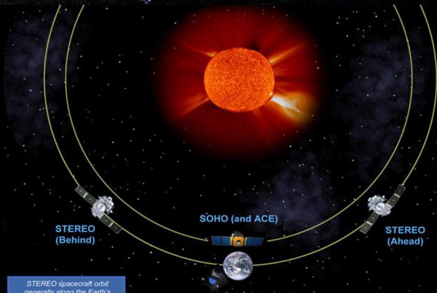
STEREO spacecraft orbit generally along the Earth's orbit path. SOHO and ACE are about 1 million miles (1.6 km) towards the sun from Earth at the Lagrangian Point L1.
