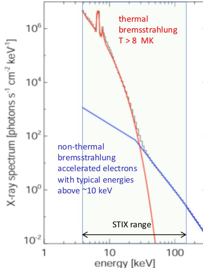
Typical X-ray spectrum of a solar flare: the red curve shows the spectrum of the hot flare loop. The blue spectrum is produced by high energetic electrons accelerated during the flare near the solar surface
